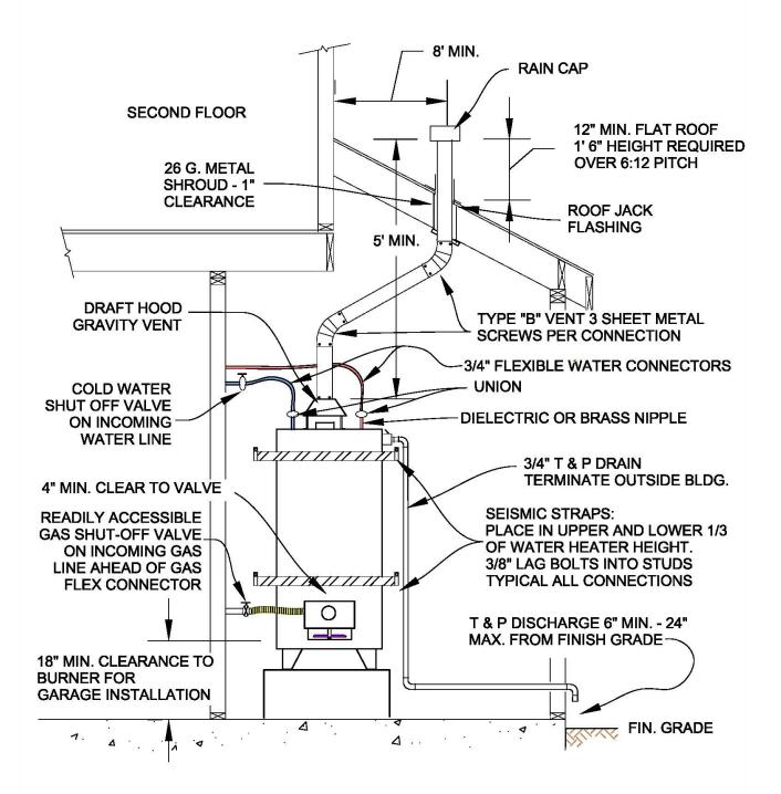
TYPICAL WATER HEATER INSTALLATION
