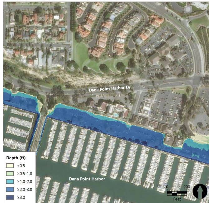
Figure 5 Flood Depths for 20-Year Waves, 6.6 Feet Sea Level Rise
