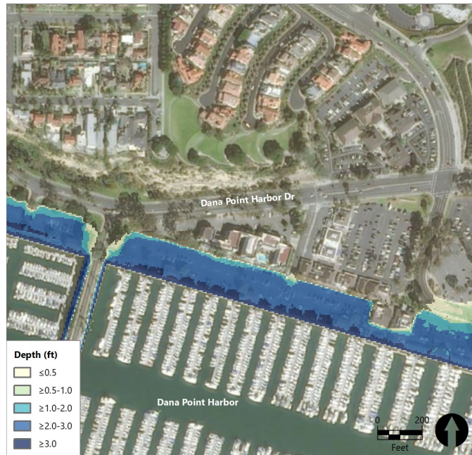
Figure 6 Flood Depths for 100-Year Waves, 6.6 Feet Sea Level Rise
