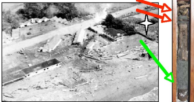
Crescent Beach Motel, Crescent City, California damaged by the 1964 tsunami. A core taken from the pond shown by the star. Deposits of sand from the 1964 and 1960 tsunamis marked by the red arrows are much smaller than the 1700 deposit marked by the green arrow.
