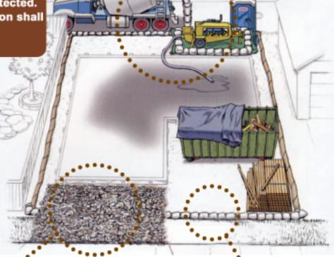
Disposal of "wet" construction materials should be handled in the washout area. This includes paint, stucco, and concrete. Use a waterproof pit (visqueen or kiddie pool, etc.) to collect and contain liquids and prevent runoff into the street and gutter. The washout area must be checked and maintained daily to ensure compliance. Washout material must be disposed of properly. Leaks must be repaired immediately.
