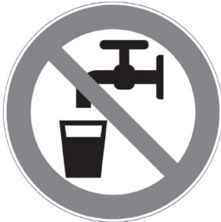
Figure F-1: Figure Required on Hose Bibbs on rainwater piping systems (Per Figure 1702.9 of the 2013 California Plumbing Code)
