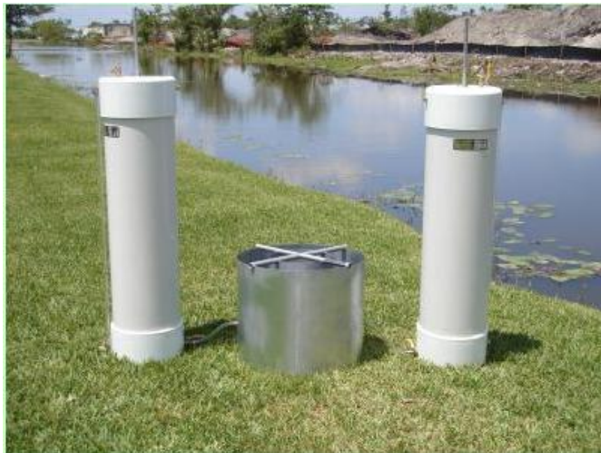
Figure D-15. Double Ring Infiltrometer Set-up with Mariotte Tubes (County of Riverside, 2011)
