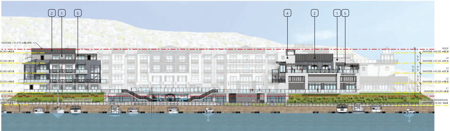
3. SOUTH ELEVATION *NOTE: F.G & F.F.E. = +24.00 FINISH GRADE & FINISH FLOOR ELEVATION FROM NAVD88
