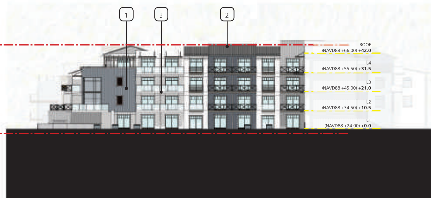
7. WEST COURTYARD ELEVATION *NOTE: F.G & F.F.E. = +24.00 FINISH GRADE & FINISH FLOOR ELEVATION FROM NAVD88
